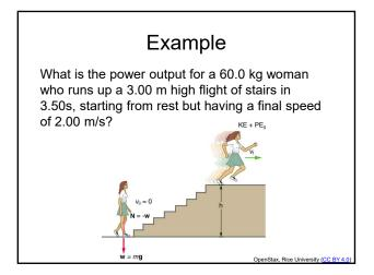
$$P = \frac{\Delta E}{\Delta t} \qquad \Delta E = \left(K_f + U_f\right) - \left(K_i + U_i\right)$$
